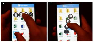
Figure 11. Hybrid touch+hover. (a) Selecting an icon with the thumb while moving a second finger into range calls up a convenient context menu. (b) With a one-handed grip, the menu gracefully degrades to a thumb-activated variant.
