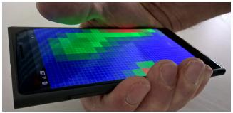
Figure 1. The pre-touch sensing modality detects multiple fingers *above* and *around* (gripping) the edges of the screen.
