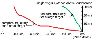
Figure 9. Example pre-touch trajectories from one pilot user for a small target (5x5 mm) versus a large target (40x40 mm). The small target requires fine adjustment, whereas the finger can "dive" to the large target with a purely ballistic motion.
